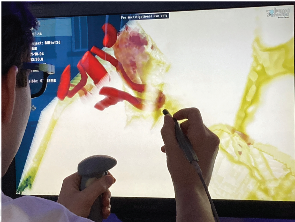
Fig. 1 Dextroscope setup. The user wears polarizing glasses and interacts with the stereoscopic, segmented patient-specific imaging data using electromagnetically tracked handheld controls, thereby seemingly reaching into the 3D simulation scenario.
